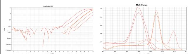
The amplification plot shows a sample with low concentration of PCV2d and Ct-values identical to nonspecific amplifications with PCV2a and PCV2 b assays. The melt curve of the sample in the PCV2d reaction though is specific for the PCV2d type. The same sample run with the PCV2a assay resulted in "primer dimer" formation at Tm <80°C, the PCV2b assay generated a small unspecific peak at Tm 90°C.
