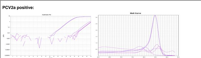
The amplification plot shows amplification curves for a PCV2a-positive sample with low Ct-values and higher Ct-values for the PCV2b and PCV2d assays run with the same sample due to unspecific amplification. The melt curve of the sample, however, is easily identifiable as a PCV2a type due to its specific peak at the expected melting point, Tm 85°C in the PCV2a reaction.
