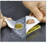
Manually pull the lower right corner back, completely exposing the protective seal. Remove the seal aby pulling the tab and discard.
